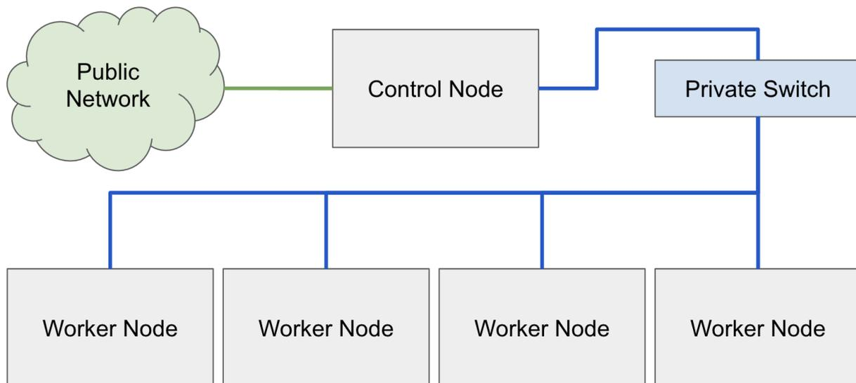
This simple topology is the foundation for creating a scalable HPC cluster resource. Even today, almost 30 years after the inception of this architecture, this is the baseline architecture that virtually all HPC systems are built to.
