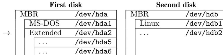
The program `activate`, that accompanies LILO, may have to be used to set the active marker on an extended partition, because MS-DOS' `FDISK` and some older version of Linux `fdisk` refuse to do that. (Which is generally a good idea.)
