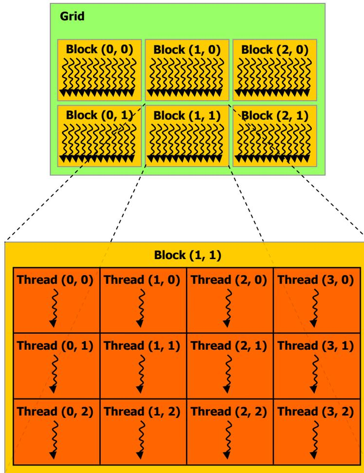
A kernel is executed over an NDRange by a grid of thread blocks.
