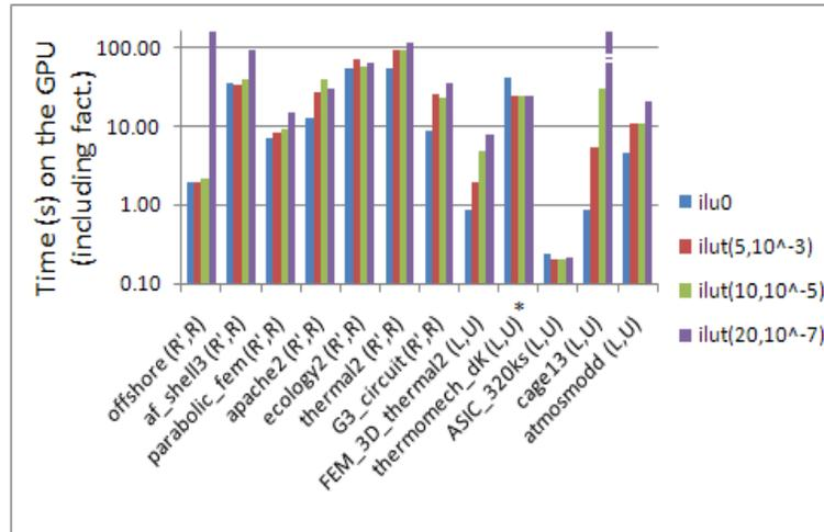
Figure 3: Performance of BiCGStab and CG with incomplete-LU/Cholesky preconditioning
